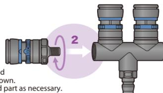
Please mout TS-2NR or TS-2WR sold separately by proper torque as shown. Please do seal treatment to thread part as necessary.
